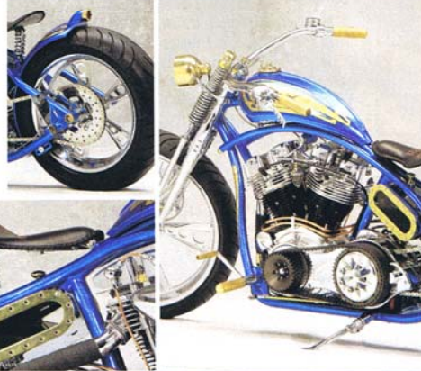
You can hardly even notice the custom-narrowed 360 Brake between the Springer legs. You never need to guess if you're low on oil with the see-through oil tank.
