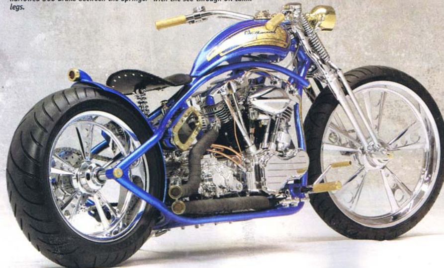
You can hardly even notice the custom-narrowed 360 Brake between the Springer legs. You never need to guess if you're low on oil with the see-through oil tank.
