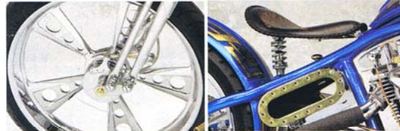
You can hardly even notice the custom-narrowed 360 Brake between the Springer legs. You never need to guess if you're low on oil with the see-through oil tank.
