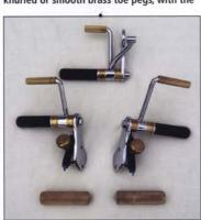
additional option of powder-coated finishes. Unlike other foot controls currently available, these ones have been designed to be compatible with regular handlebar grips. This move means that users can match the controls to those used on the bike's bars, or use rubber or Neoprene grips that can offer a level of vibration damping.
