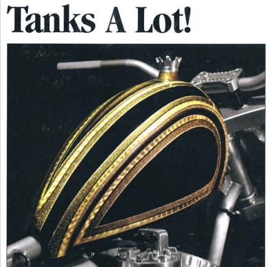
The popular "Pinche" tank is finally being made available to the cashpaying public courtesy of Gard Hollinger from LA County Choprods. Designed to mount "Frisco" style (high on the backbone of the frame), this trick fuel cell features an inset panel on each side. The one-piece bottom also features sunken mounts. A choice of gas caps and its location, as well as the style and location of the
