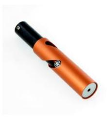
Gard Hollinger of <u>LA County Choprods</u> has redesigned his internal throttle assembly. This new unit now uses a "slide plunger" with two thread-in double ball bearing pin and bearing assemblies. In addition the new aluminum "outer tube" has two spiral travel grooves and has been lengthened in order to close the inner end of the travel grooves to eliminate the possibility of misshaping the tube when your handgrip set screws are tightened.
