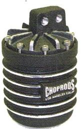
50s, these filters have been adapted for use on motorcycles. Cast, heattreated and machined from aluminum, they are available in three finishes: natural, polished and black wrinkle with polished highlights.
