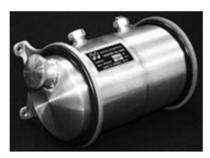
This "Side Mount" battery box is designed to allow a standard Softail size battery to be mounted on the right side above the transmission. The box mounts in three places and uses rubber isolated mounts for vibration resistant installation and includes
