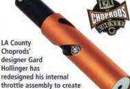
throttle assembly to create an improved version for 2009. The revised design now uses a 'slide plunger' with two thread-in double ball bearing pin and bearing assemblies, along with a new aluminum outer tube that has two spiral travel grooves, which has been lengthened in order to close the inner end of the travel grooves to eliminate the possibility of mi-shaping the tube when the handgrip set screws are tightened. The finish on the assembly has been changed too and it is now hard anodized.
